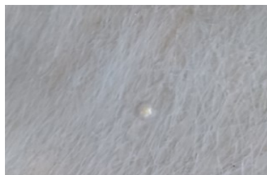
Figure 1. Gel lumps on the surface of the material.
