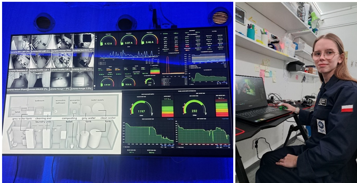
Figure 5. Round-the-clock monitoring of mission participants and microclimate parameters in the habitat, as well as all resources, including oxygen, drinking water, grey water, waste, etc. Architecture student Natalia Ściora during the PEGASUS mission (photo archive: Klaudiusz Fross, Natalia Ściora).
