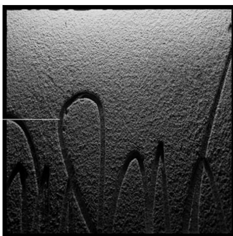
Figure 9. Image of the coating layer thickness relative to the sheet of paper in the form of an indentation.
