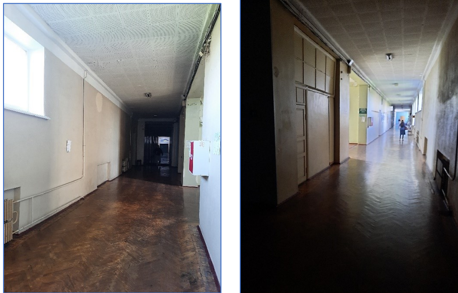
Figure 4. Corridor entrances: a well-lit area ( E = 257 lux) and a dimly lit area ( E = 17 lux).
