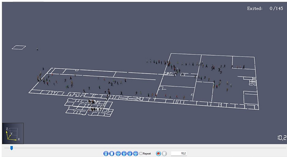
Figure 14. Simulation 3 – evacuation with some emergency exits unavailable.
