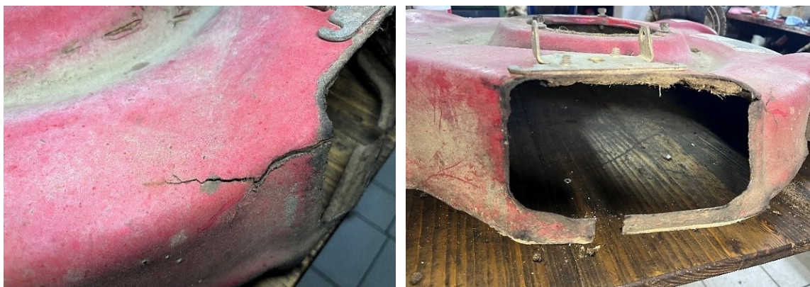
Figure 1. Damage to the mower body as a result of dynamic loads.
