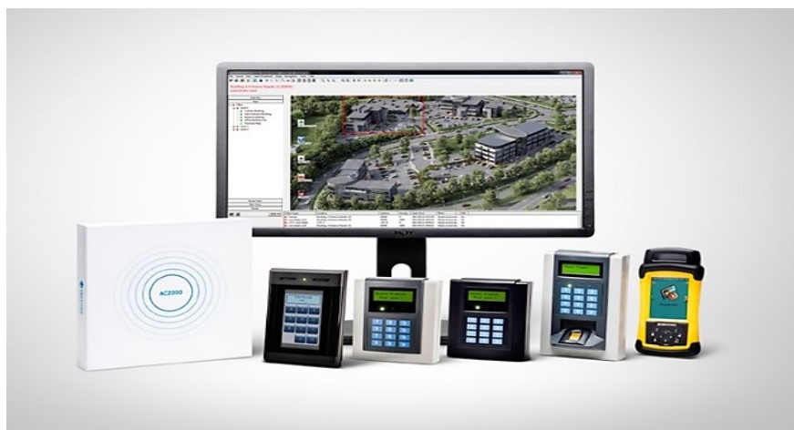
Figure 1. AC2000 Airport system components.
