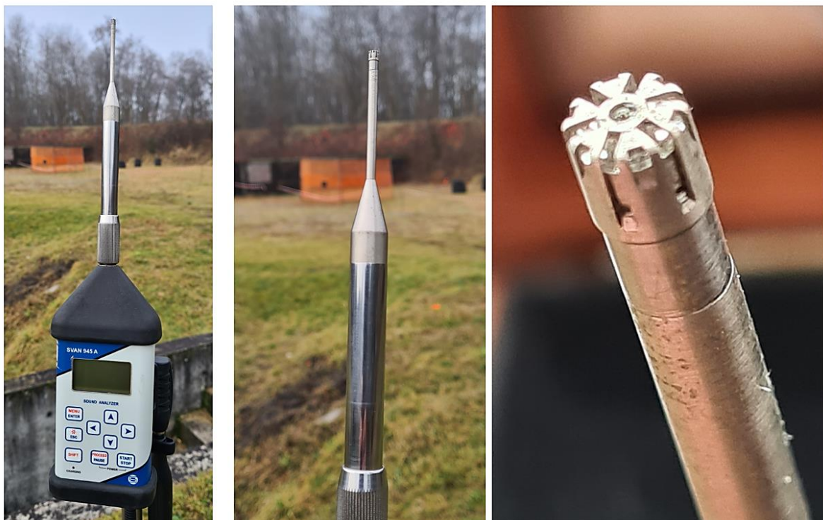
Figure 3. Measurement set for recording impulse signals.
