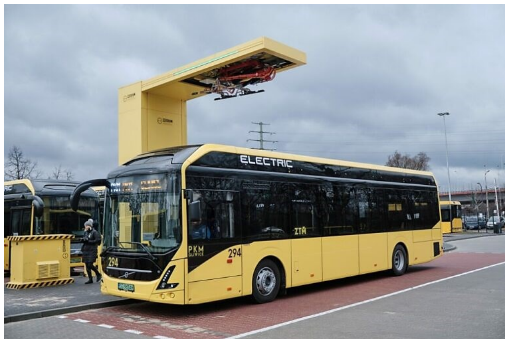
Figure 4. Electric bus preparing for charging with a high power pantograph connection in the terminal station.
