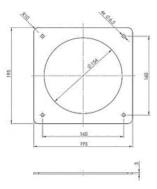
Figure 2. Housing flange.
