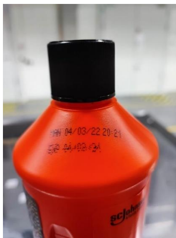
Figure 11. Example of a photograph with a bad expiry date printed on it.
