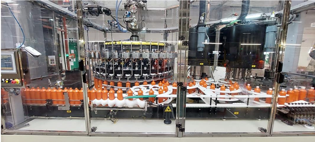
Figure 4. Pouring and capping machine.
