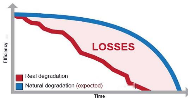
Figure 1. Decrease in efficiency due to degradation of photovoltaic panels.
