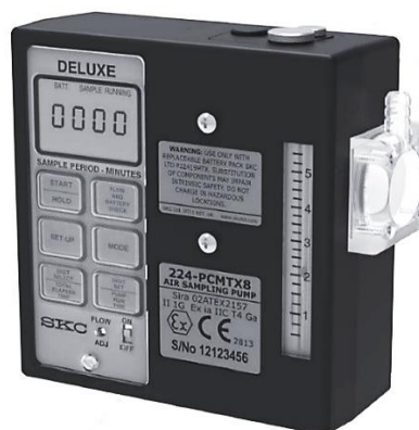
Figure 2. Type 224-44 MTX individual aspirators used in environmental studies.
