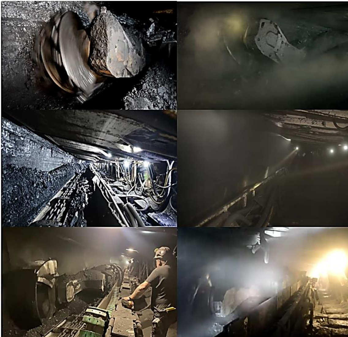
Figure 4. Dust in the coal face area of the G-1 mining division of X Mine.
