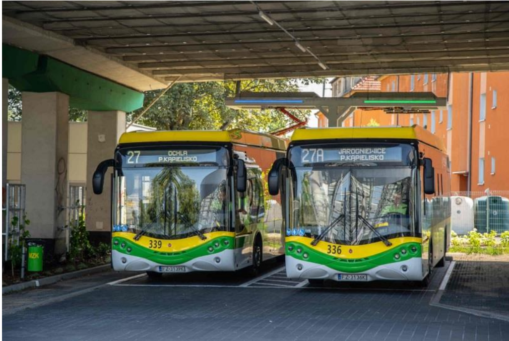
Figure 1. Buses charging at the transfer centre.
