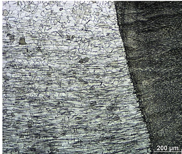
Figure 3. Structure of correct dissimilar weld (above 316L on the left, DOCOL 1200 M on the right). Sample Q11, electrolytic etched with 10% oxalic acid.
