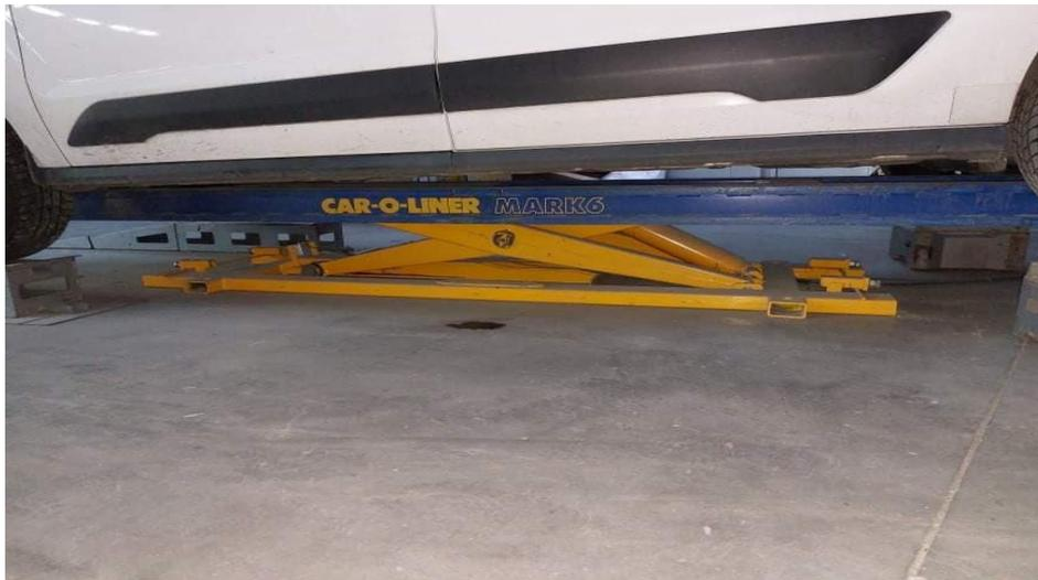
**Figure 6.** Car Frame Straightening Machine.
