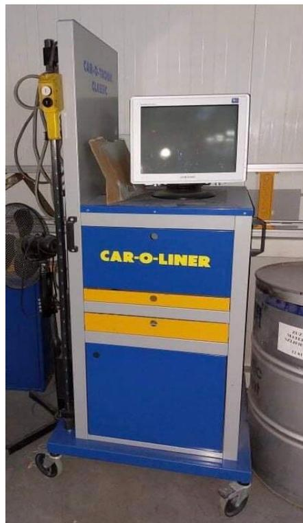
**Figure 7.** Computer Operating the Car Frame Straightening Machine.
