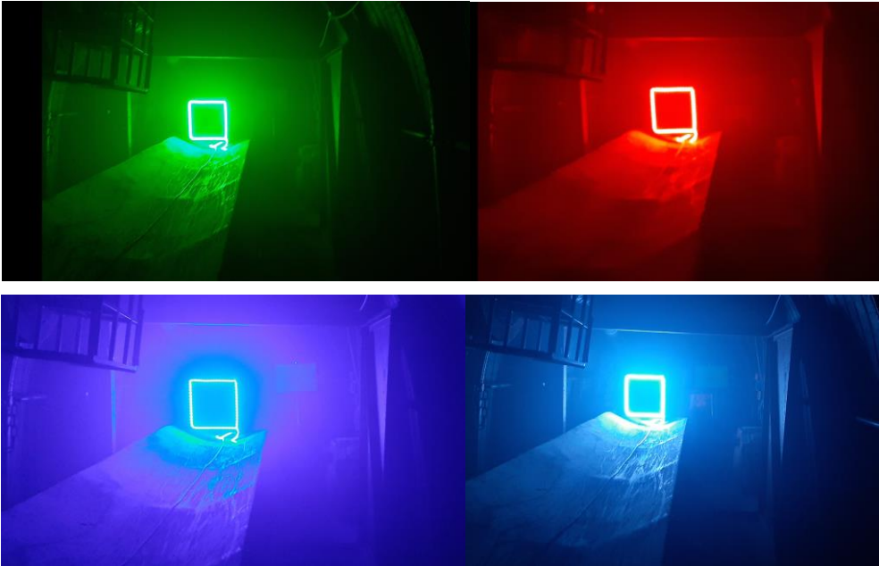
Figure 7. Observation of the square shaped sign, a the distance of 5 m.
