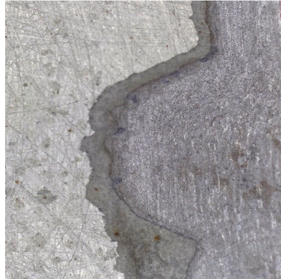
Figure 9. Specimen AW-6060 with alkyd varnish – 630 hours.
