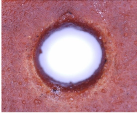
Figure 14. Round hole in specimen AW-6060 with alkyd varnish +40% brick dust – 630 hours.
