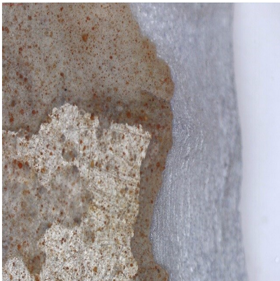
Figure 10. Specimen AW-6060 with alkyd varnish +10% brick dust – 630 hours.
