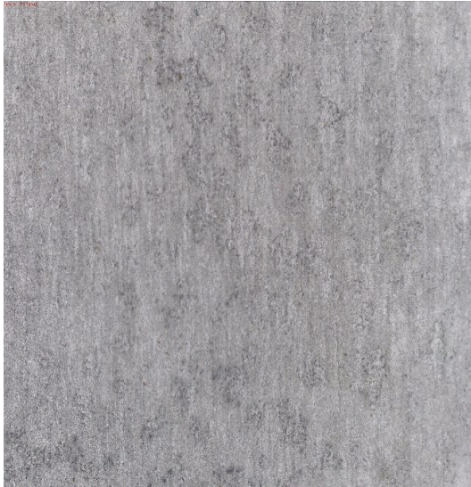
Figure 8. Specimen AW-6060 without corrosion protection coating – 630 hours.
