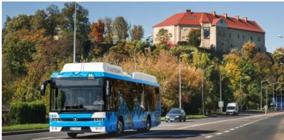
Figure 4. A zero-emission hydrogen-powered bus SANCITY 12LFH. Adopted from Trans Expo Kielce 2021: Solaris displays four zero-emission buses.
