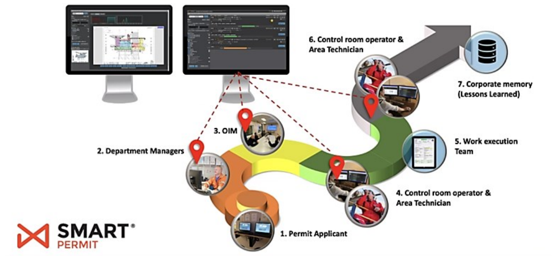
Figure 7. Electronic PTW System workflow. Source: eSmart permit user guide.
