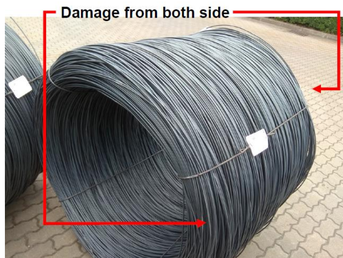
Figure 1. Unloaded wire rod with damage on both sides. Adapted from: Company materials.
