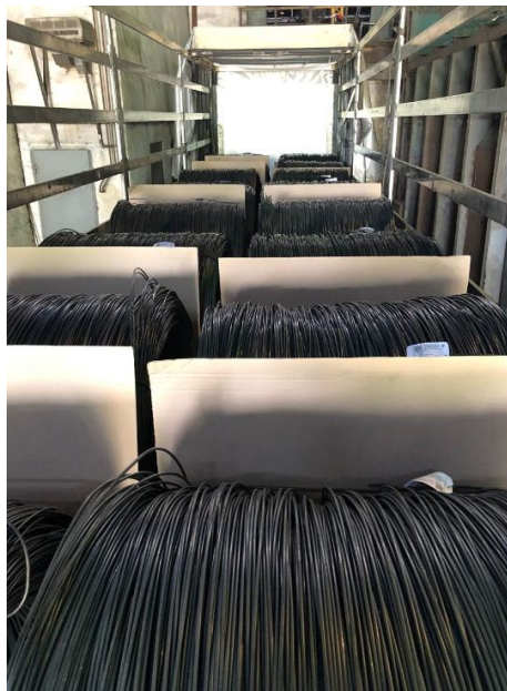
Figure 6. Carton boards among the wire rod coils, picture taken during the transport. Adapted from: Company materials.
