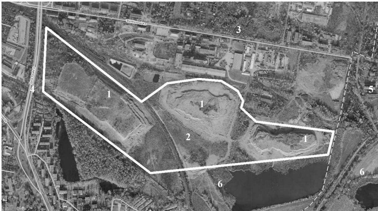
**Figure 1.** Bird's-eye view of the area to be redeveloped. 1. Heaps of solid excavation waste, 2. Active railway line no. 132, 3. national road 94, 4 national road 79, 5 Administrative border of Bytom and Chorzów, 6. „Żabie Doły” nature and landscape complex (own elaboration based on Geoportal Bytom, 2020).
