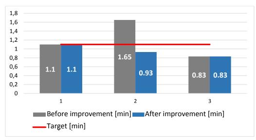
Figure 9. Line balance before and after improving the process.
