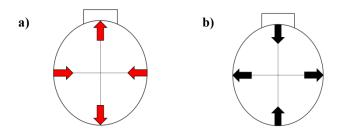
**Figure 6.** Direction of a) welding deformations on the pipe material during cooling, b) forces on the pipe material during expansion with an oval tool.
