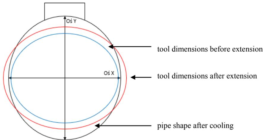
**Figure 5.** Sketch of the tool dimensions before and after expansion with respect to the pipe contour.
