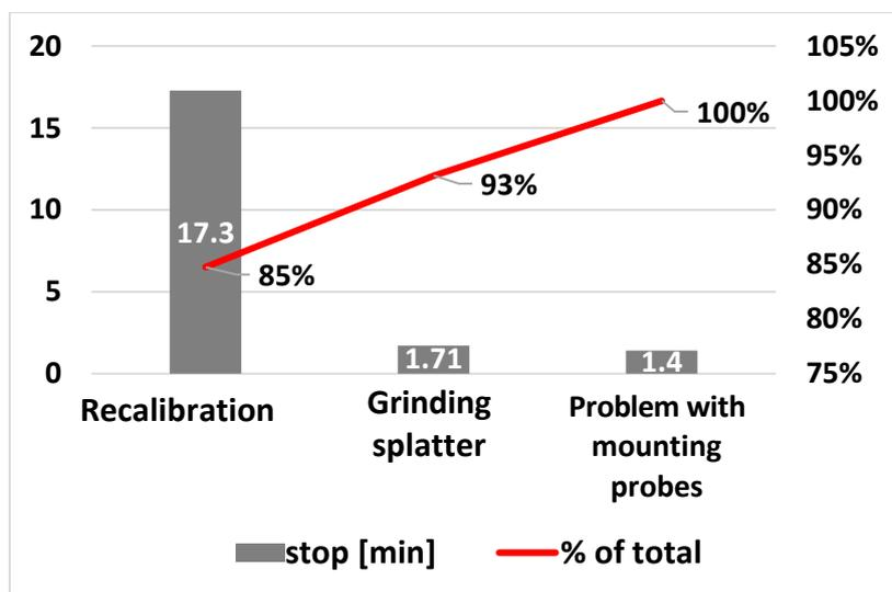
Figure 3. Pareto Chart of losses during run at rate.
