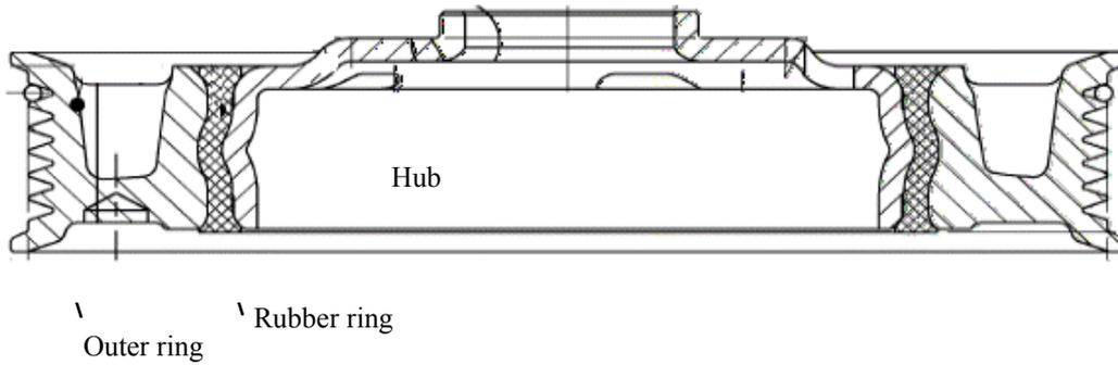
**Figure 1.** Structure of a model vibration damper.
