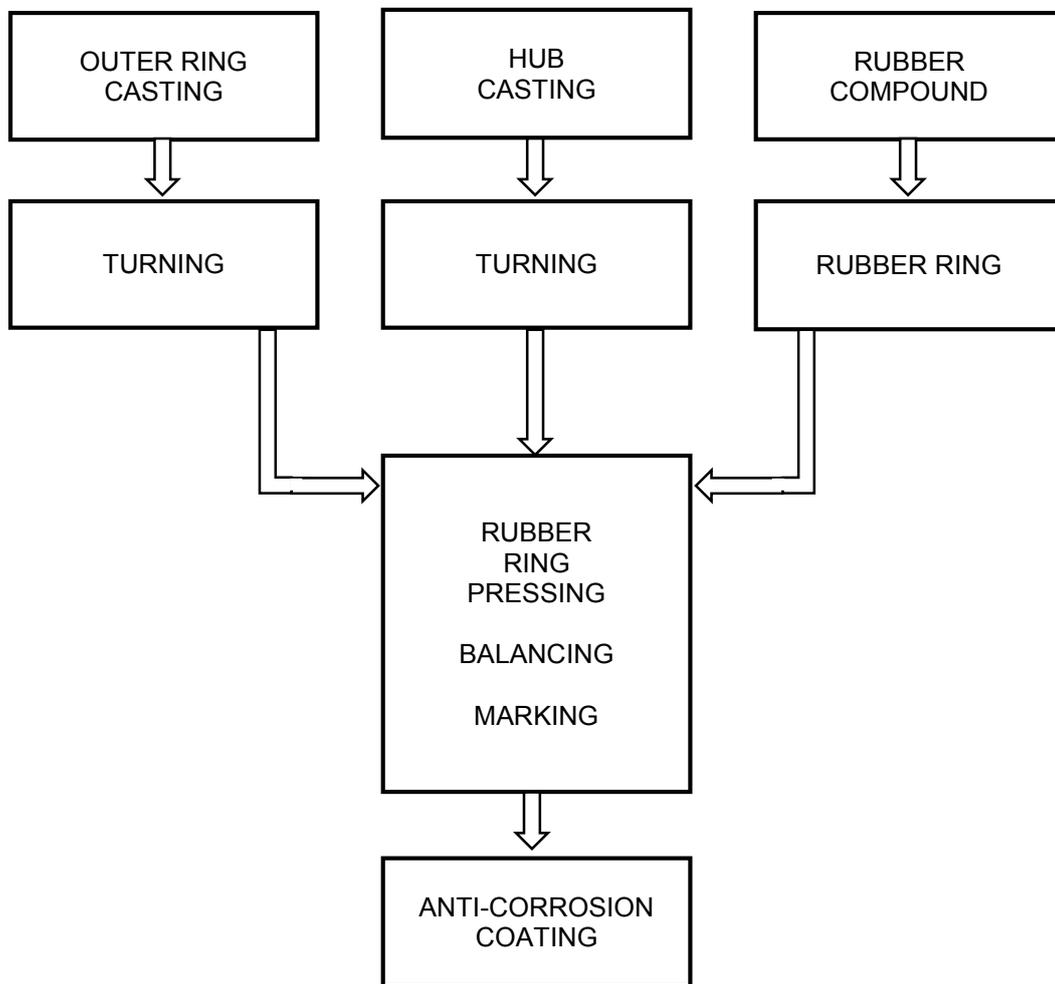
**Figure 2.** A block diagram of the vibration damper production process.
