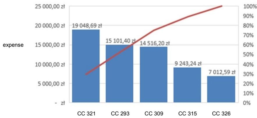
**Figure 8.** Pareto diagram – costs of non-conforming products by codes.
