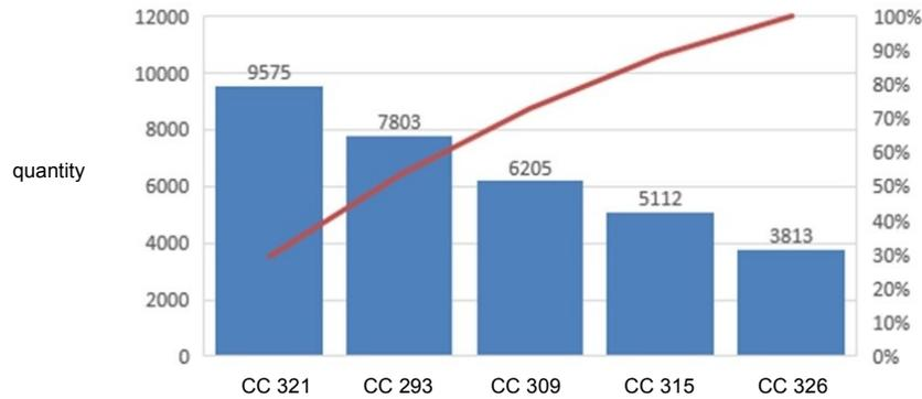
**Figure 7.** Pareto diagram – quantitative amount of non-conforming products by codes.
