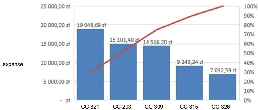
**Figure 6.** Pareto diagram – costs of non-conforming products by CC.
