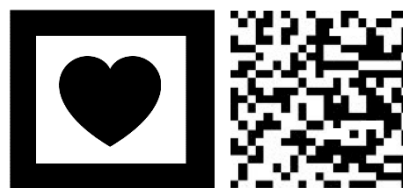
Figure 2. Examples of markers used for image detection. One white hole is visible on the left marker. On the right there is a binary maker, there are many white holes and strong edges that are used to quickly calculate the acceptance criteria.
